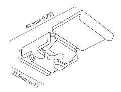
New C-Track Ceiling Holder (C010) Click System Ceiling Mount for Convenient Installation Purpose.
