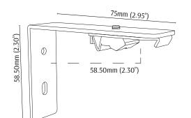
New C-Track Wall Holder (C009) Click System Wall Mount for Convenient Installation Purpose.
