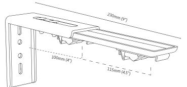
Ripple Double Track Wall Holder for C-Track (RDH-CT01) Developed to carry Wave Curtains.
