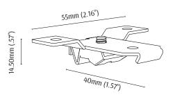
C-Track Ceiling Mount (C003) MS, Powder Coated, Click System Fittings for Ceiling installations.
